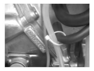
The serial number can be found stamped on the engine block above oil dipstick. It is visible when the service access door is removed.
