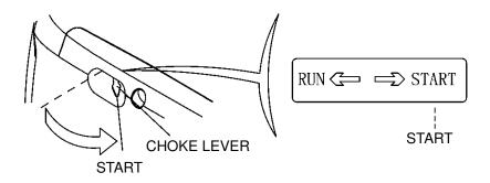
3. Pull the starter grip until resistance is felt then pull the starter grip briskly toward the arrow as shown below.
