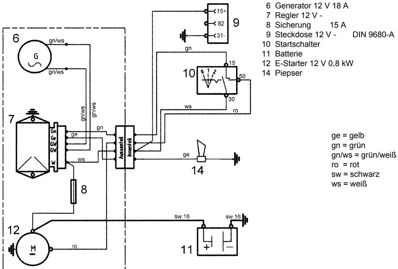
**Elektroplan 5900 Taifun Benzin-Motor B&S Vanguard 18 HP (5900 231, -232)****Sicherheitsschaltung**
